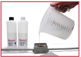
The mixing of the Power Gel is effected with the spatula in the measuring cup in the desired amount with a mixing ratio of 1:1. Non-required material in the PE bottles can be stored for up to 12 months for further use. The discharge aid of the cup allows for a clean cast of branch and connection boxes.
