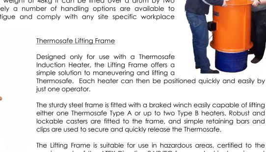
requirements of the ATEX Directive 94/9/EC for non-electrical equipment and Machinery directive 98/37/EC. The Lifting Frame can be supplied in two base widths; a wider width to incorporate drums on pallets, or a standard unit for applications where this is not necessary.
