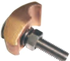
For clamping earth cable to flat metal. Needs only one spanner as head of bolt has square shank to prevent turning. Standard bolt grips 6mm bar.
