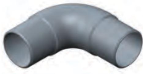
BUSLIGHT™ welded elbows are used to create horizontal or vertical angles within busbar tube assemblies. Installation is normally made via Metal Inert Gas (MIG) welding. Standard angles are 30, 45, 60 and 90 degrees. Other angles are available on request.
