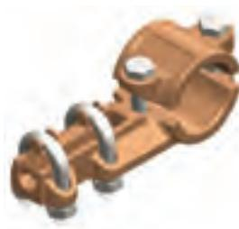
The BUSSIGN™ D-T is designed for connecting copper busbar tubes and copper flexible conductors in a tee configuration. The advantage of this design is that each model of this type of connector can accept a wide range of flexible conductor sizes. Contact surfaces of the connectors and conductors must be thoroughly cleaned before assembly and use of Electropar PLP's white Joint Seal compound which is specifically designed for copper conductors and bolted joints is recommended.
