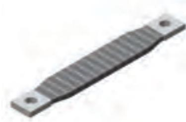
Series "F" flexible braid connectors consist of one or more tinned copper flat braids. Specially formed tinned copper ferrules are swaged onto the ends of the braids under high pressure to form solid rectangular terminals. Short Time Rating - Based on maximum current density being below 115 amps per mm<sup>2</sup>. Time period basis, 3 seconds.
