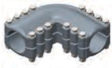
BUSSIGN™ bolted elbows connect busbar tubes of the same size. The standard angles are 30, 45, 60 and 90 degrees, but specially manufactured angles are available on request. Contact surfaces of the busbar tubes and the connector must be thoroughly cleaned before the joint is assembled using PLP's jointing compound specially designed for high current / high voltage bolted electrical connections.
