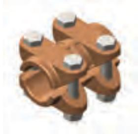
The BUSIGN™ D-ST coupler is designed for connecting same sized copper busbar tubes. This is a heavy duty connector recommended for high current connections because unlike U bolt type connector designs both halves of the connector carry current. Contact surfaces of the connectors and conductors must be thoroughly cleaned before assembly and use of Electropar PLP's white Joint Seal compound which is specifically designed for copper conductors and bolted joints is recommended.
