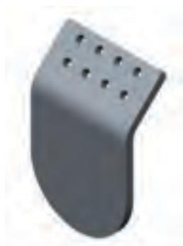
BUSLIGHT™ welded end terminals allow flexible conductors or primary equipment to be connected to a busbar tube. In straight configuration, the terminal palm sits exactly on the centreline of the busbar tube. When used as a busbar support, it can be attached to either the top or the bottom of the substation primary equipment terminal. The EPBWET-135 is installed via Metal Inert Gas (MIG) welding to the busbar tube and can be used as a bus support as well as a terminal palm.
