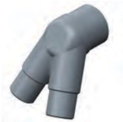
The EPWVC vee connector is used in combination with BUSLIGN™ welded, bolted or welded/bolted hybrid tee connectors to create rigid busbar A frame connections. This style of welded vee connector sets the A frame at a 60 degree angle relative to the low perpendicular busbar. When using the EPWVC, the type of tee connector at the bottom of the A frame should be the 75 degree angled EPBWTC, EPBBTC or EPBWTC.
