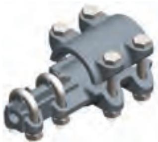
A heavy duty tube-to-conductor end connector. The adjustable tap takes a large range of conductors which may be clamped before attaching to tubular bus.
