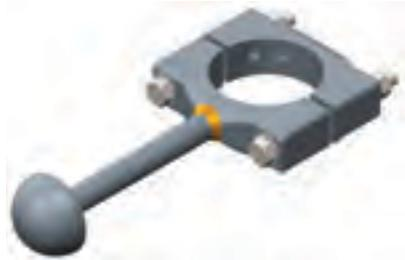
BUSSIGN™ bolted earth ground points are designed to be bolted to busbar tubes so that a temporary earth lead or ground lead can be applied to the busbar tube. The dome shaped head of the earth point is designed to eliminate corona and Radio Interference Voltage (RIV) while at the same time providing a solid stop at its end to eliminate the risk of the earth lead or ground lead sliding off the earth point when the lead is being applied via hotstick.
