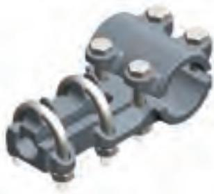
A heavy duty tube-to-cable tee connector. The adjustable tap takes a large range of cables which may be clamped before attaching to tubular bus.
