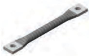
Series "R" flexible braid connectors consist of one or more tinned copper round braids with specially formed tinned copper ferrules swaged onto the ends of the braids under high pressure to form solid rectangular terminals.
