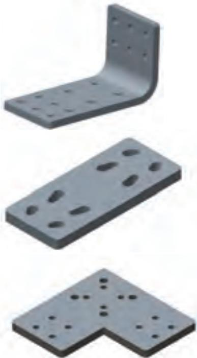
Adapter plates are customized for specific applications. Manufactured from 6000 series high conductivity aluminum alloy user specified terminal palm designs, lengths, widths, shapes and angles are commonplace. Standard thickness for adapter plates are 12mm, 16mm, 20mm and 25mm. Contact Electropar PLP for specific requirements and current ratings.
