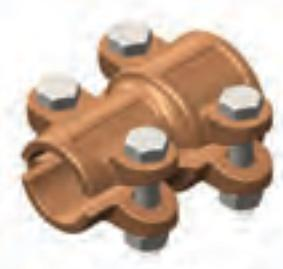
The BUSSIGN™ D-RT coupler is designed for connecting different sized copper busbar tubes. This is a heavy duty connector recommended for high current connections because unlike U bolt type connector designs both halves of the connector carry current. Contact surfaces of the connectors and conductors must be thoroughly cleaned before assembly and use of Electropar PLP's white Joint Seal compound which is specifically designed for copper conductors and bolted joints is recommended.
