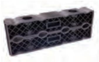
Cable Blocks fasten cable diameters from 12 mm up to 32 mm. By means of 2 block parts, 4 cables can be fastened alongside each other. Additional cables are able to be fastened alongside each other by coupling the block parts together using the standard dovetail connection. Contact PLP with specific requirements and conductor diameters.
