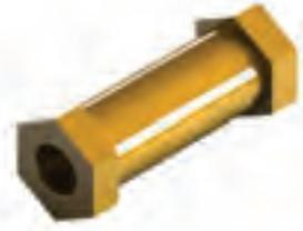
Earthing stubs are made from high purity brass, able to carry fault currents up to 40kA for 0.5 seconds or equivalent and suitable for connection of earthing devices onto structures.
