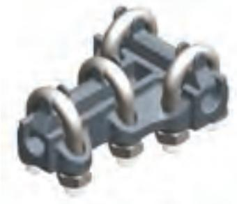
A high strength aluminium alloy tee connector for all aluminium and SCA run and tap conductors. U-bolts and nuts are stainless steel.
