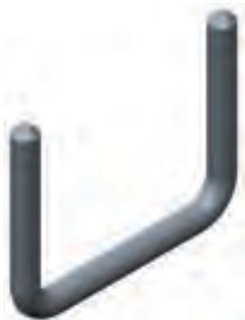
BUSLIGHT™ welded earth ground points are designed to be welded to busbar tubes so that a temporary earth lead or ground lead can be applied to the busbar. Manufactured from extruded aluminium alloy round bar, the EPBWES suits any sized Aluminium busbar tube. Installation is made via Metal Inert Gas (MIG) welding. If stirrup lengths or heights other than standard are required, specify in the PLP catalogue number as illustrated below.
