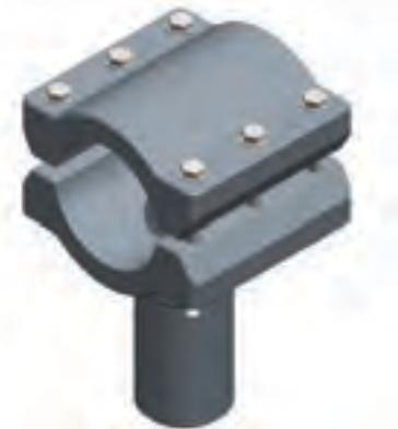
The EPBWTC90 bolted run welded tee connector is an ideal way of making a reliable, maintenance free midspan connection between two busbar tube conductors. Most often used for connections between high and low perpendicular busbar tubes, the Metal Inert Gas (MIG) welded side of the connector can be completed in a factory or workshop environment so the final assembly simply bolts together on site.
