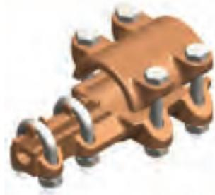
The D-E allows a single flexible conductor to be connected to the end of a copper substation busbar. This connector has been specifically developed as a range taking fitting so that each model of connector can accommodate a variety of copper flexible conductor sizes. For installation, contact surfaces of the connector and copper busbar tube must be thoroughly cleaned before assembly. Use of Electropar PLP's white Joint Seal compound specifically designed for copper bolted joints is recommended.
