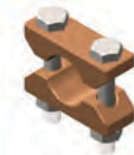
The BUSSIGN™ D-PTC is designed for connecting copper busbar tubes to switchgear terminal palms that have 4 holes at 50mm centres and M12 bolts. Two D-PTC connectors are required per termination. Contact surfaces of the connectors and conductors must be thoroughly cleaned before assembly and use of Electropar PLP's white Joint Seal compound which is specifically designed for copper conductors and bolted joints is recommended.
